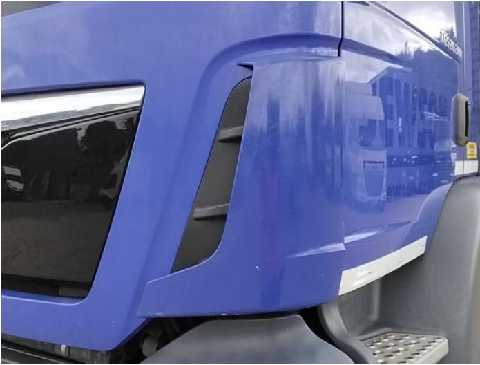
9: Wing nsf Chipped Multiple Chips
